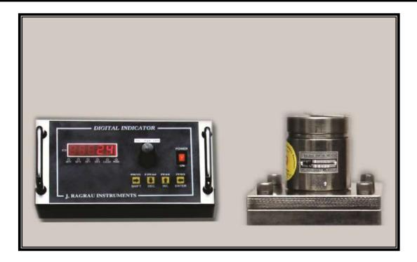
**JRAGRAU INDUSTRIES** offers low cost, high accuracy torque wrench verification system the instruments are easy to operate user friendly. These are available in various ranges up to 2000 Nm.
